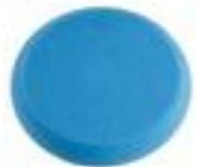
Sponge of a medium-hard, coarse foam structure and high resistance to tearing. With setback velour for assured polishing and as a centering aid. Particularly for weathered, dull paints and for scratches in combination with the fine polishing compound.
