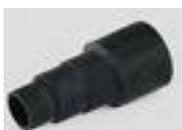
Universal adapter with 32 mm thread inside for universal connection of machines with 25-32 mm Ø extraction connection with 32 mm suction hose (without clip attachment), adapter can be trimmed to 3 different diameters.
