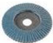
Ideal for flap-grinding metals, stainless steel, alloyed and non-alloyed steel, light metals, non ferrous metals, construction steel and cast iron. Removing welding spots and beads, processing welding seams, breaking and rounding edges. High material removal rate, guarantees effortless working without filling pores.
