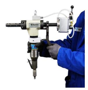
The US25CA is a powerful. durable. reliable and versatile portable tube and pipe beveling & facing machine. The PROTEM US25CA will perform repeatable high quality weld end preparations on virtually all materials including mild, chrome, stainless steel, duplex, super duplex, copper-nickel alloy steel, inconel, P91, aluminium, copper, exotic alloys, etc...
