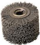
Impregnated with sanding grits. Flexible, interspersed plastic brushes. For deburring, cleaning, roughing and smoothing. (Also suitable for wood, brushing applications and removing fibres.) Needed is one piece plus distance ring set (order no. 250.522).
