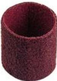
For removing minor damage, scratches, tarnish, flash rust, scale and dirt. Removing tarnish at welds without heat distortion at thin plates. For grinding, cleaning and finishing stainless steel, steel, titanium alloys, light metals, non-ferrous metals and plastics.
