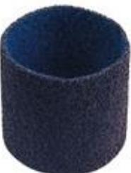
For removing minor damage, scratches, tarnish, flash rust, scale and dirt. Removing tarnish at welds without heat distortion at thin plates. For grinding, cleaning and finishing stainless steel, steel, titanium alloys, light metals, non-ferrous metals and plastics.
