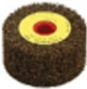
Flexible polishing wheel made of sanding grit-impregnated nylon web with a keyway. Two wheels are required (for 50 mm wide fleece only). Achieves effective surface finishes on stainless steel, copper, aluminum, brass, etc. Also ideal for cleaning oxidized coatings and smoothing plastic and wood.
