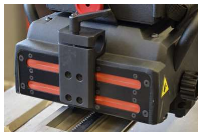
Silicone covers protect against dirt and spatter
