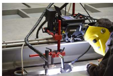
TIG welding of titanium plate
