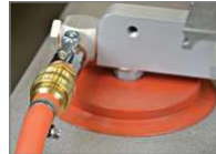
Cut-off valve (for entry vacuum unit) ZWR-0541-10-01-30-0
