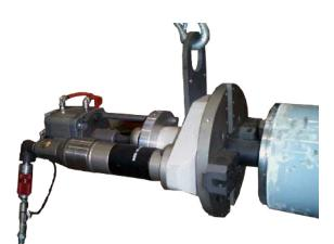
The portable id mount PROTEM US40CA tube and pipe beveling machine is powerful, durable, reliable and versatile. The US40CA covers Ø ranging from 43mm (1.692") to 219mm (8.622"). The standard tool plate will accept multiple tool bits, allowing up to four simultaneous machining operations which may include 30°, 37°30. 45° bevels with or without land, J-bevels, compound bevels, facing, counterboring operations,cutting tubes to length and removal of weld joints from heat exchanger tubes.
